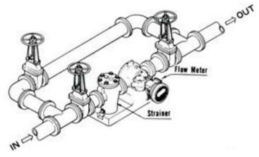
1) It is recommended that when setting up pipe work for meter installations a bypass line be included in the design. This provides the facility for a meter to be removed for maintenance without interrupting production. (see figure above)
